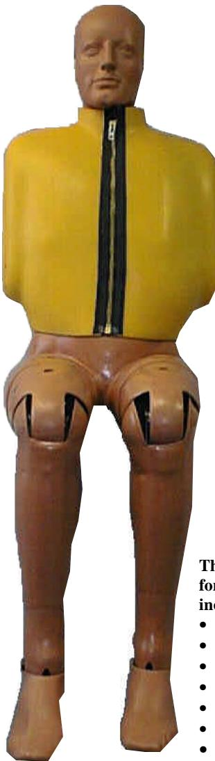
The Side Impact Dummy (SID) was originally developed under NHTSA contract to the University of Michigan. This program was undertaken to develop a manikin capable of producing human-like responses when impacted in the lateral direction during an automotive side impact crash. This Title 49 CFR Part 572, Subpart F device is the only ATD specified as meeting the requirements of FMVSS Standard No. 214. (Side Impact Protection).
