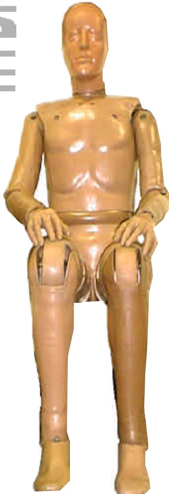
The Hybrid II 50<sup>th</sup> Percentile Adult Male Test Dummy was developed by General Motors in 1972 to assess lap / shoulder belt systems. The Hybrid II was the first dummy designed to achieve acceptable repeatability and good durability.
