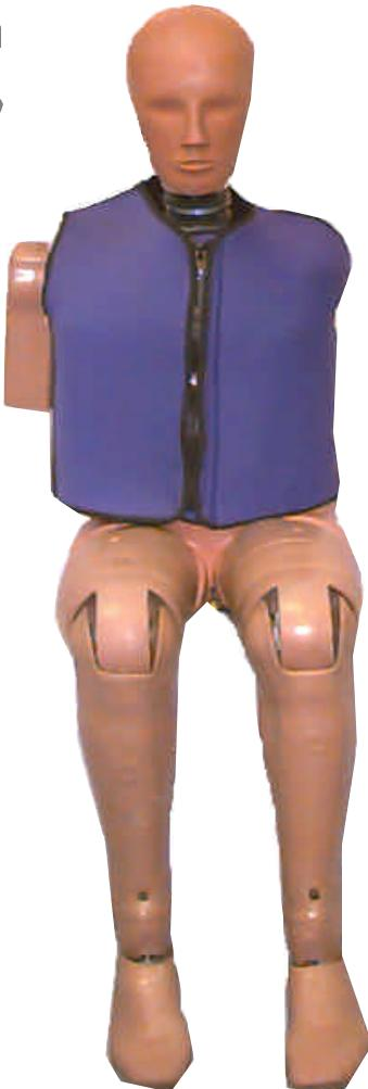
The BioSID (Biofidelic Side Impact Dummy) was developed through the cooperative efforts of the Side Impact Dummy Task Force (an SAE Committee). This program was undertaken to improve the impact responses of side impact mannequins by meeting the biofidelity requirements developed by TC22/SC12/WG5. Although not required for certification use under title 49CFR, Part 571(214) or 572, the BioSID has proven to be an effective R&D tool.
